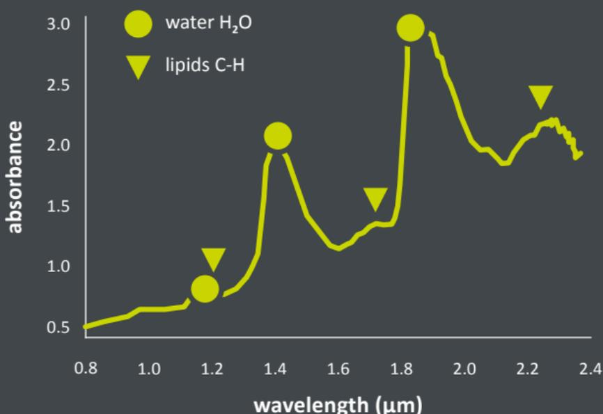
Near-infrared (NIR) spectroscopy utilizes the molecular characteristics of relevant biomarkers such as water and lipids to provide accurate and reliable information about hair and skin conditions. The direct measurement on a molecular level enables the simultaneous but independent assessment of different biomarkers.
